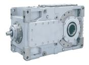
The new bevel helical series from Bonfiglioli optimises superior performance with compact dimensions and flexibility. The several options that can be selected from the catalogue facilitate customization to meet specific application requirements. Gear case from nodular cast iron guarantee rigidity in all circumstances while gears, integrally ground finished on their profile, ensure quiet and vibration-free operation even in the harshest conditions.
